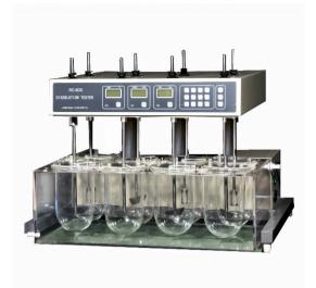
RC-8DS Tablet dissolution tester, LCD display
